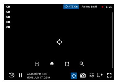
The camera's PTZ controls are overlaid on the video and manual pan and tilt controls are enabled. For more information on using manual pan and tilt controls, see *Moving a PTZ Camera* on the next
